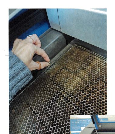
Choose the cutting bed when you are cutting wood, fabric, cardboard, paper, etc, or when etching on light materials like flat glass from picture frames.
