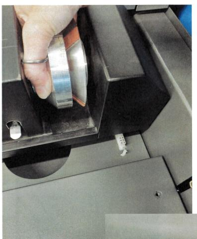
You will probably need to turn the ULS on before changing to the Rotary for glasses, vases, and powder-coated mugs, because you will probably need to lower the cutting bed so the rotary will fit beneath the laser lens carriage.
