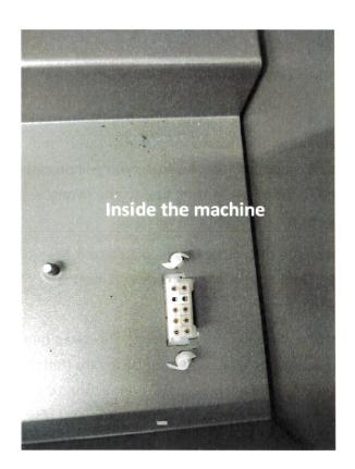
When changing any of the beds, you will find an 8-prong plug inside the Laser, and a corresponding plug on the bottom of the bed. These must connect securely for the software to allow you to print.
