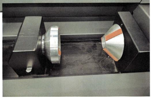
Once the rotary is installed, you can unlock the left side and slide it open.
