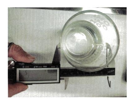
When measuring for the rotary, measure the diameter of your glass or mug, as the ULS wants to know how high above your material it needs to be, not how thick the glass is .
