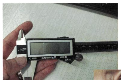
Turn the calipers on and make sure it is on inches if your design is in inches, and that it starts at 0". (If it is not at zero, use the zero-out button while it is closed to reset.)
