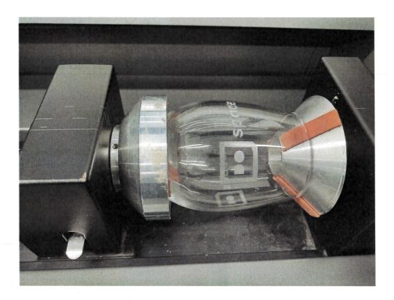
A warning about HANDLES: You can engrave things with handles, but keep in mind that the rotary turns your mug while it etches. It may hit either the carriage housing or the bottom while turning if your image that is being etched is wide. It happens. This can squish pictures and words, or knock the entire cup out of alignment during the engraving.
